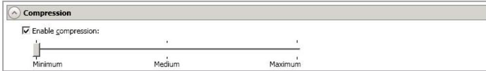
To help reduce the amount of bandwidth needed to transmit Double-Take data, compression allows you to compress data prior to transmitting it across the network. In a WAN environment this provides optimal use of your network resources. If compression is enabled, the data is compressed before it is transmitted from the source. When the target receives the compressed data, it decompresses it and then writes it to disk. You can set the level from **Minimum** to **Maximum** to suit your needs.
