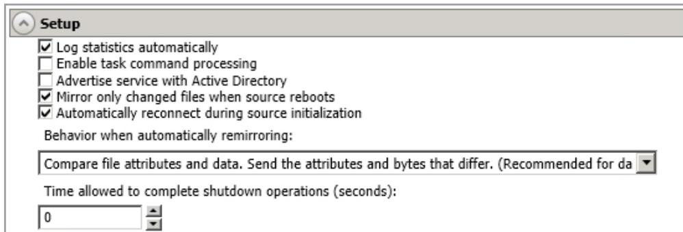
Server setup properties indicate how the server will act on startup and shutdown.
