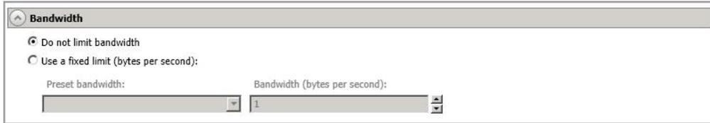
Bandwidth limitations are available to restrict the amount of network bandwidth used for Double-Take data transmissions. When a bandwidth limit is specified, Double-Take never exceeds that allotted amount. The bandwidth not in use by Double-Take is available for all other network traffic.
